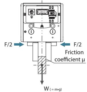
\*While the conveyable workpiece weight increases with the static friction coefficient, select a model offering grip force of 10 to 20x or more for safety purposes.
