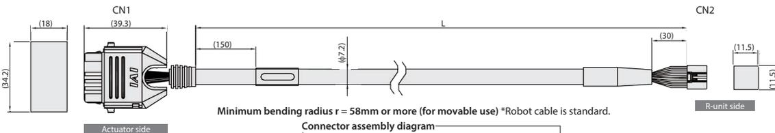
Minimum bending radius  $r = 58\text{mm}$  or more (for movable use) \*Robot cable is standard.
