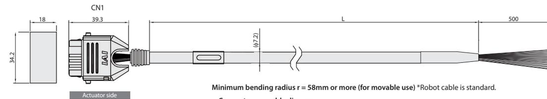
Minimum bending radius  $r = 58\text{mm}$  or more (for movable use) \*Robot cable is standard.
