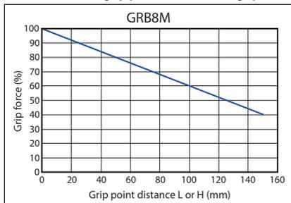
(Note) Shows grip force of overhang position when maximum grip force is set to 100%. The results may differ due to the rigidity of the finger attachment used.
