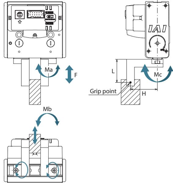
\*The load point above indicates the position where the load is applied to the finger.
