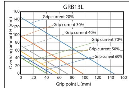
(Note) Use beyond the limited range will cause excess moment to operate on the finger sliding part and interior mechanisms, negatively affecting operation life.
